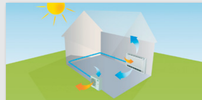
In summer, heat energy is released from inside to outside (only possible with AquaFree).
